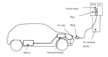
In mode 1, 2 and 3 the charging takes place through the converter in the vehicle (AC from the charging station to DC in the vehicle battery) and the charging process is being controlled by the vehicle. The capacity of the converter determines how much of the available charging capacity of the charging station can be utilized.
