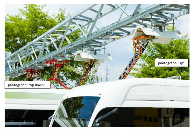
The 'top down'-pantograph is often applied on a start-, stop or endpoint of a public transport bus route. At those places the bus is being charged in a very short time also called 'opportunity charging'. This type of pantograph lacks a direct physical communication connection between the ACD and the vehicle. Therefore a WLAN/WIFI connection is used which requires special attention for cyber security.
