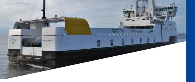
The **e-ferry** is capable of carrying 30 vehicles and 200 passengers and is powered by a battery "with an unprecedented capacity" of 4.3MWh, according to Swiss battery maker Lechanché which provided the system.
